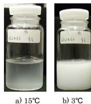
Fig. 5 Thermo-sensitivity of microspheres sampled at different conversions
